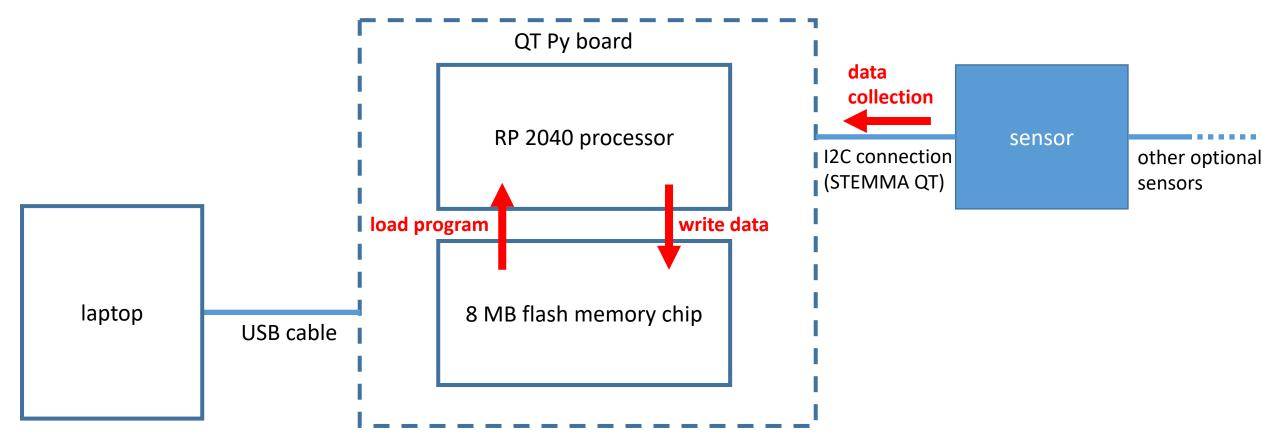
The processor can write to the memory chip.
